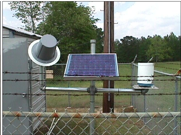
Figure 5-2 Typical Field Installation of Precipitation Gage
